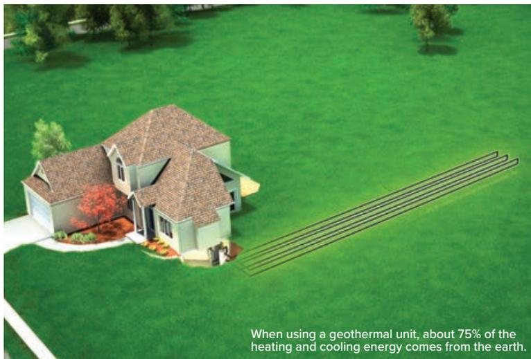
When using a geothermal unit, about 75% of the heating and cooling energy comes from the earth.
