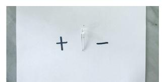
Attach the LED: Tape the LED bulb to the top edge of the index card, with wires pointing down. Leave plenty of space at the bottom of the wire to connect with the aluminum foil conductor. Label the wires directly on the card (+ and -).
